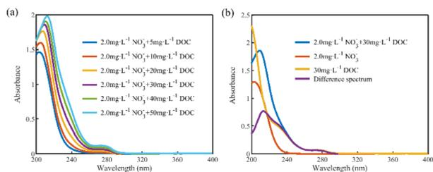
Fig. 3 (a) Absorption spectra of nitrate and DOC mixed solutions (take  $2 \text{ mg L}^{-1}$  nitrate as an example). (b) Difference spectra between mixed solutions and nitrate solutions (take  $2 \text{ mg L}^{-1}$  nitrate as an example).
