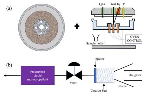
Fig. 4 Schematic diagrams of (a) batch catalytic reactor structure. Reprinted with permission from ref. 84. Copyright 2003 American Institute of Aeronautics and Astronautics, and (b) self-designed simulation thruster. Reprinted with permission from ref. 90. Copyright 2014 Springer.
