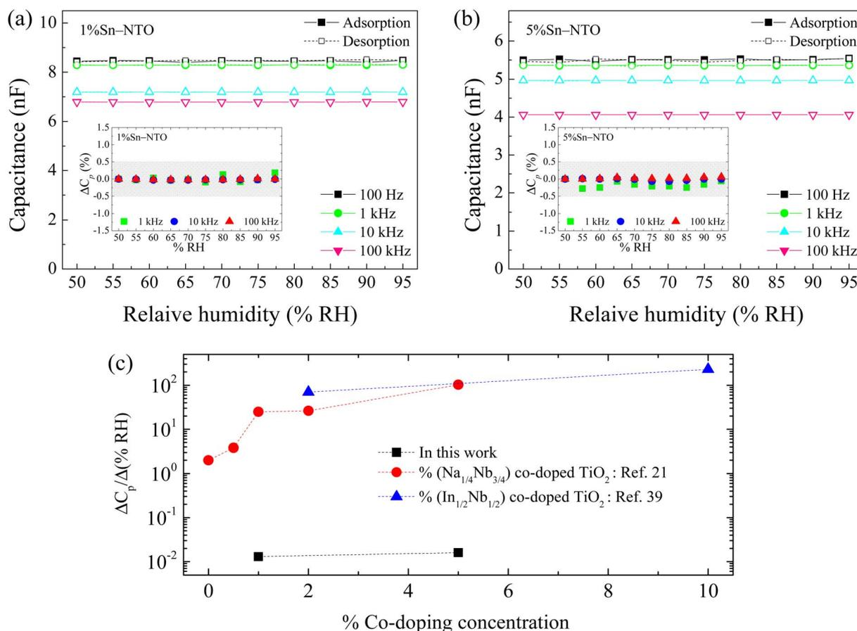
Fig. 6 Relative humidity dependence of  $C_p$  at 25 °C and several frequencies for (a) 1% Sn-NTO and (b) 5% Sn-NTO; their insets show the  $\Delta C_p(\%)$ . (c) Comparison of  $C_p$ -humidity sensitivity of Sn-NTO with (In + Nb) and (Na + Nb) co-doped  $\text{TiO}_2$  ceramics.
