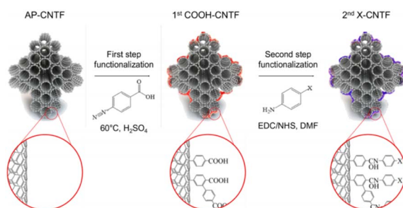
Fig. 28 Schematic representation showing the surface treatment of CNTF proposed in this work. 134
