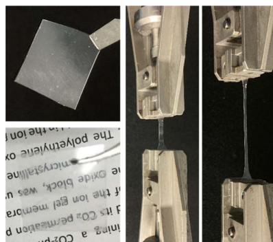
Fig. 2 Examples of the prepared ion gel membrane composed of [Emim][C(CN) 3 ] and Pebax 1657.
