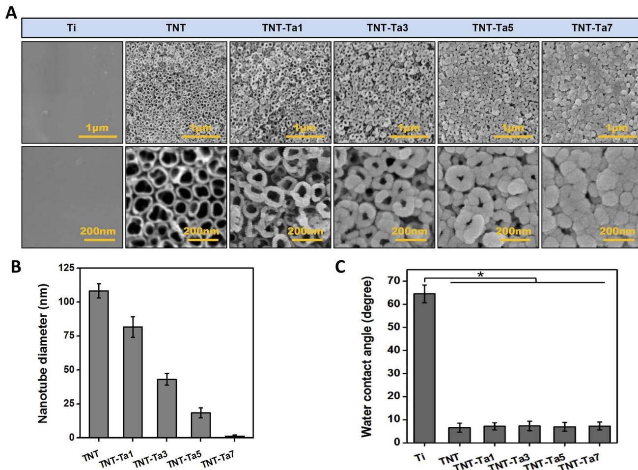
Fig. 1 (A) The SEM image of different specimens (Ti, TNT, TNT-Ta1, TNT-Ta3, TNT-Ta5, and TNT-Ta7) ( $n = 6$ ). (B) Corresponding statistical analysis of the diameters of different nanotubes. (C) Water contact angle measurements of different specimens (Ti, TNT, TNT-Ta 1, TNT-Ta3, TNT-Ta5, and TNT-Ta7) ( $n = 6$ ),  $*p < 0.05$ .
