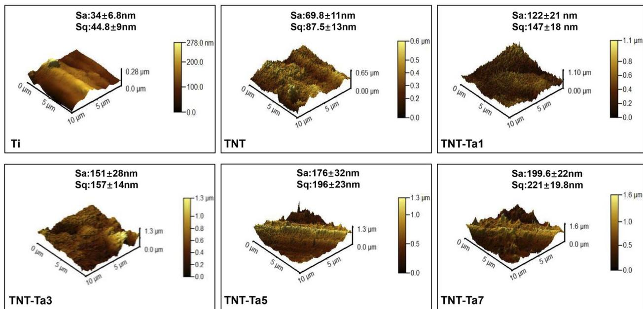
Fig. 2 AFM images showing the average roughness (Sa) and root mean square deviation of the surface (Sq) of different substrates ( $n = 6$ ).
