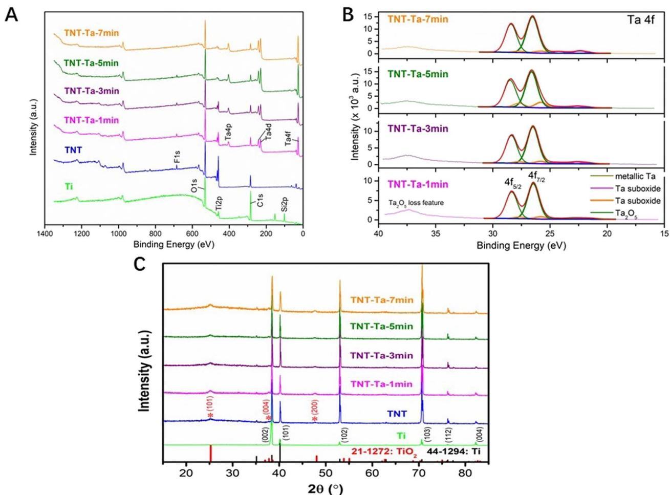
Fig. 3 (A) XPS analysis of different samples ( $n = 6$ ), (B) detailed spectrum for Ta XPS analysis ( $n = 6$ ). (C) XRD showing the crystalline structure of different samples (Ti, TNT, TNT-Ta 1, TNT-Ta3, TNT-Ta5, and TNT-Ta7) ( $n = 6$ ).
