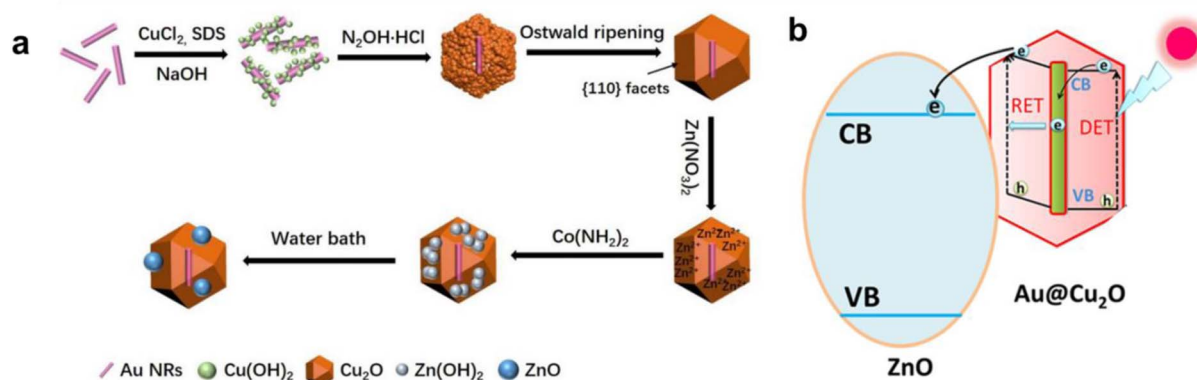
Fig. 1 Composite diagram (a) and electric transition diagram (b) of the Au@Cu 2 O@ZnO ternary heterojunction.
