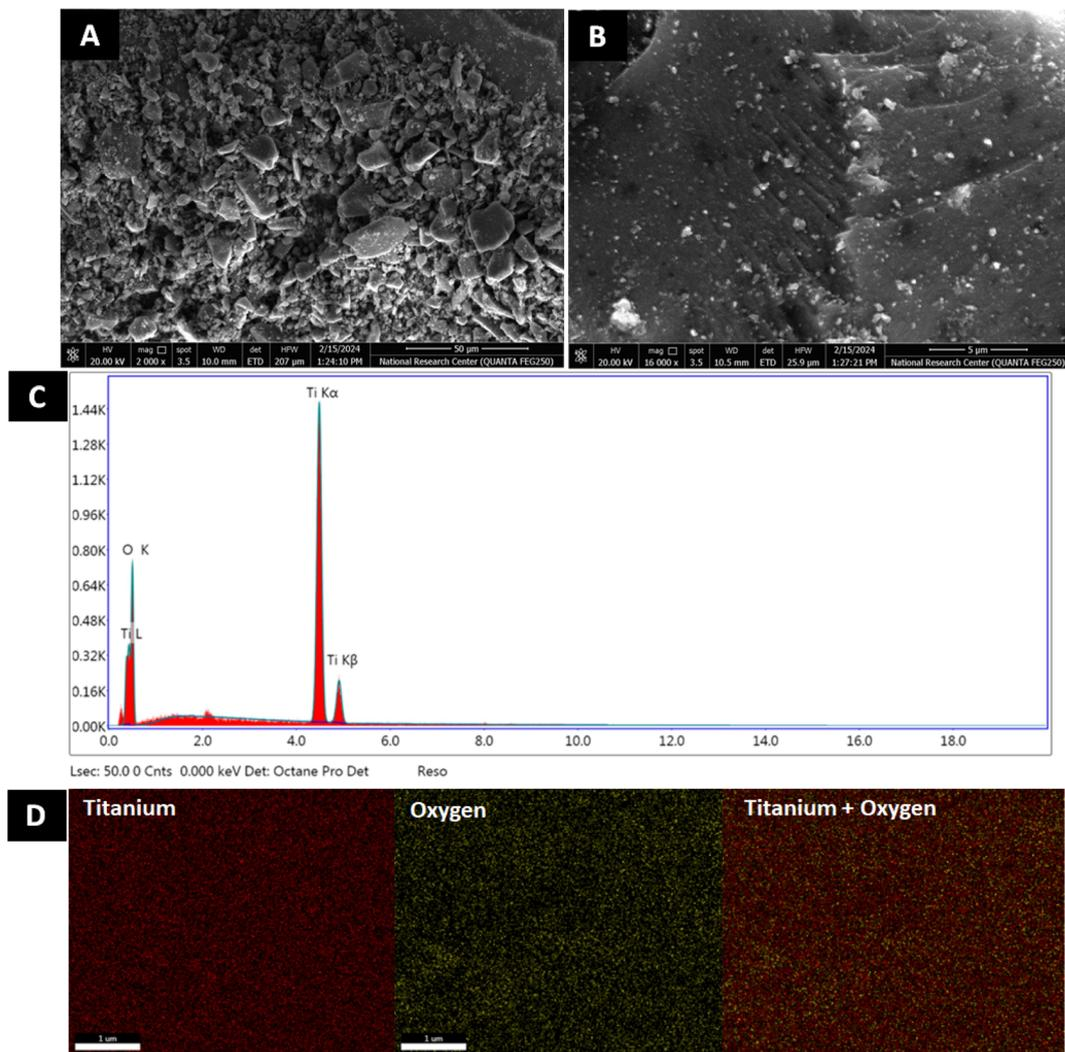
Fig. 3 Morphological and structural analysis of TiO<sub>2</sub> NPs. SEM of TiO<sub>2</sub> NPs at (A) 50 μm and (B) 5 μm, (C) EDX profile and (D) EDX mapping analysis of TiO<sub>2</sub> NPs.
