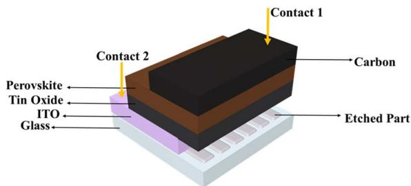
Fig. 2 Perovskite photodetector cell configuration.
