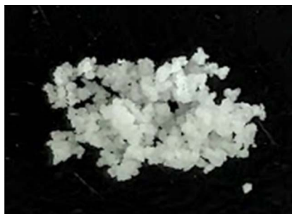
Fig. 3 FD product obtained through freeze-drying, comprising solid-state cubic \text{NH}_3(\text{cr}) as the main constituent.
