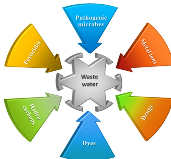
Fig. 1 Various types of wastewater contaminants.
