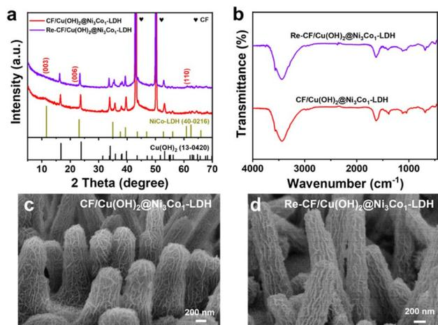
Fig. 6 (a) XRD patterns and (b) FT-IR spectra of CF/Cu(OH)<sub>2</sub>@Ni<sub>3</sub>Co<sub>1</sub>-LDH and Re-CF/Cu(OH)<sub>2</sub>@Ni<sub>3</sub>Co<sub>1</sub>-LDH. SEM images of (c) CF/Cu(OH)<sub>2</sub>@Ni<sub>3</sub>Co<sub>1</sub>-LDH and (d) Re-CF/Cu(OH)<sub>2</sub>@Ni<sub>3</sub>Co<sub>1</sub>-LDH.
