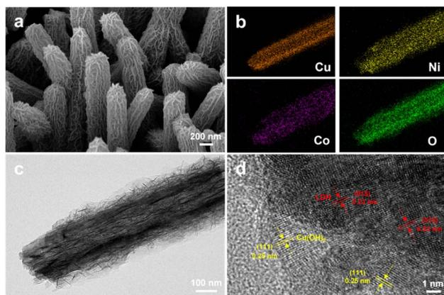
Fig. 2 (a) SEM image, (b) elemental mappings, (c) TEM image and (d) HRTEM image of CF/Cu(OH)<sub>2</sub>@Ni<sub>3</sub>Co<sub>1</sub>-LDH.
