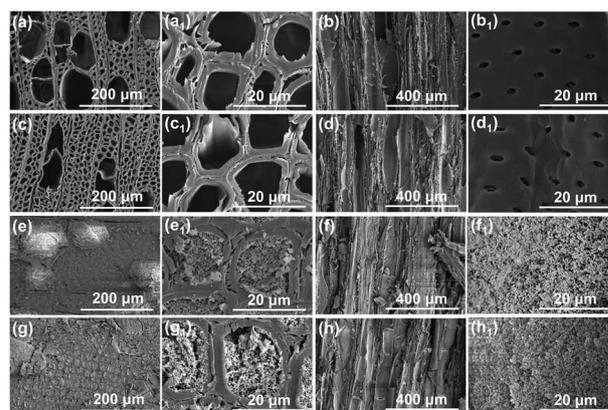
Fig. 3 Micromorphology of wood samples in cross-section and longitudinal sections: (a, a<sub>1</sub>, c, c<sub>1</sub>, e, e<sub>1</sub>, g, g<sub>1</sub>) micromorphology of the cross-section of original wood, IEMA wood, PDVB wood, and IEMA-PDVB wood, respectively; (b, b<sub>1</sub>, d, d<sub>1</sub>, f, f<sub>1</sub>, h, h<sub>1</sub>) micromorphology of the longitudinal section of original wood, IEMA wood, PDVB wood, and IEMA-PDVB wood, respectively.
