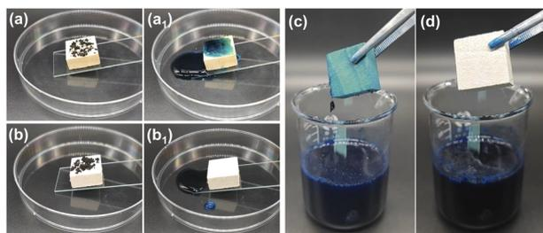
Fig. 7 Self-cleaning and antifouling properties: (a, a<sub>1</sub>) images of the self-cleaning process on original wood surfaces; (b, b<sub>1</sub>) images of the self-cleaning process on IEMA–PDVB wood surfaces; (c, d) antifouling properties of the original wood and IEMA–PDVB wood.
