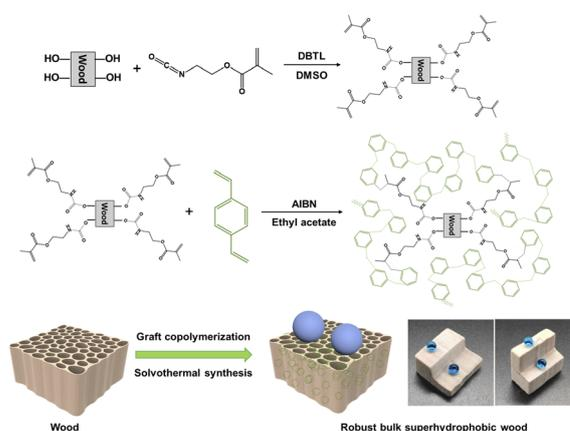
Fig. 1 Preparation process and reaction mechanism of robust superhydrophobic wood.
