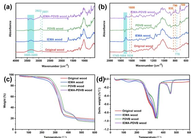
**Fig. 5** Chemical components: (a and b) FTIR spectra of original wood, IEMA wood, PDVB wood, and IEMA–PDVB wood; (c and d) TG and DTG curves of original wood, IEMA wood, PDVB wood, and IEMA–PDVB wood.
