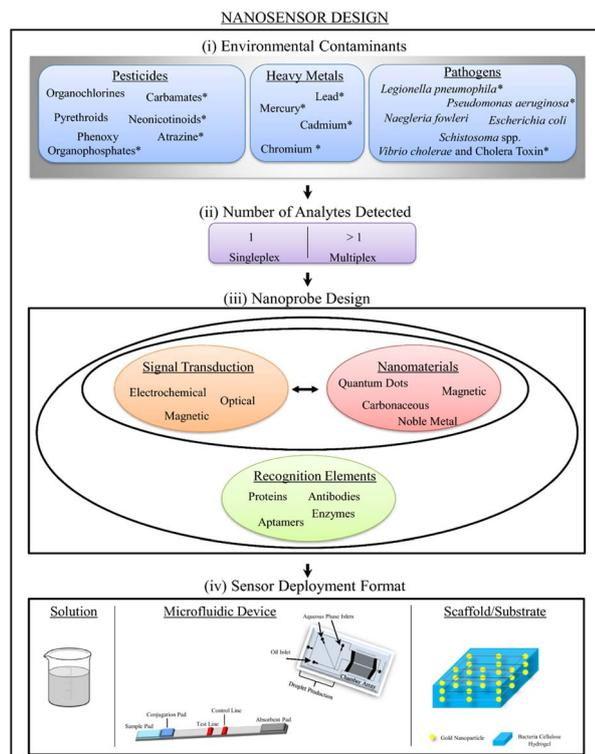
Fig. 14 Schematic illustration of nanosensor design, including ambient contaminants, detected analytes, probe design, and deployment format. Reproduced with permission from ref. 201, copyright 2024, *J. Nanobiotechnol.*
