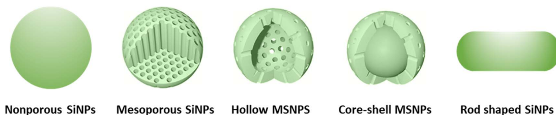
Fig. 6 Various types of silica nanoparticles with different shape and surface morphology. Each nanoparticles exhibited unique properties which can be used for specific applications.
