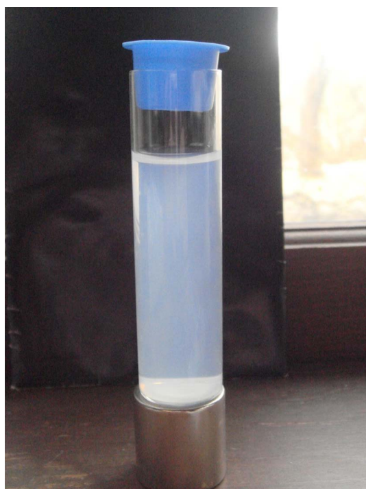
Fig. 16 The final magnetic separation of anatase titania in 0.01 N HCl exposed to ambient light. The levitated particles are fully dispersed in the solution on day 43.
