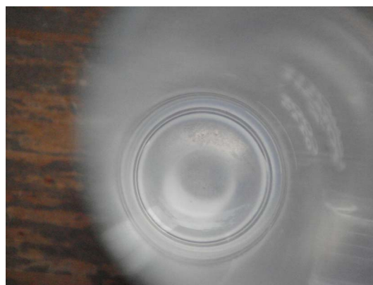
Fig. 18 Magnetic separation of anatase titania dry powder residue after the removal of the 0.01 N HCl and evaporation of the remaining liquid on day 43. The powder at the base of the tube, with an empty circular region, is evidence that the particles were pushed out of the strongest part of the magnetic field as they settled.
