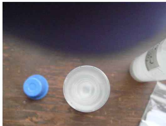
Fig. 17 A view of the powder circles created by settling particles before the solution was removed on day 43. The concentric rings demonstrate how the settled particles were rejected by the strongest portion of the magnetic field during settling.
