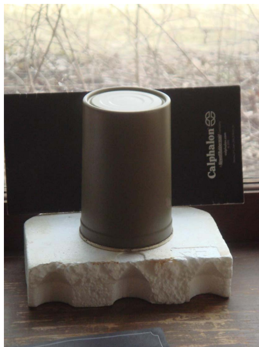
Fig. 21 Metal cup set-up used to exclude ambient light during non-magnetic settling on day 53.
