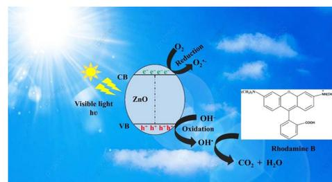
**Fig. 8** Photocatalytic degradation mechanism of RhB by porous ZnO coral-like nanoplates under simulated sunlight.
