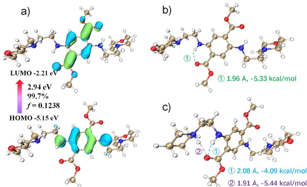
Fig. 3 The frontier molecular orbitals (HOMO and LUMO) of the  $S_1$  state of DMSS-AM in water during the vertical excitation process (a); the molecular configuration, hydrogen bond length, and hydrogen bond strength of DMSS-MA in water under neutral (b) and acidic (c) ground conditions.
