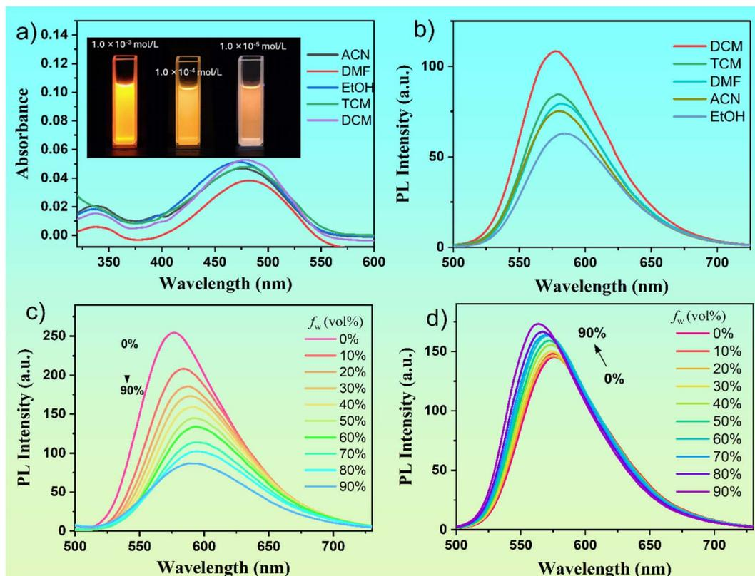
Fig. 1 Absorption (a) and emission (b) spectra of DMSS-AM in different organic solvents, fluorescence emission spectra of DMSS-AM in THF/H<sub>2</sub>O mixed solvents with different water contents (c), and in THF/*n*-hexane solutions with different concentrations (d). The concentration of DMSS-AM is  $1 \times 10^{-5}$  M; The photo inserted in 1a shows the luminescence photo of DMSS-AM at different concentrations under 365 nm UV excitation.
