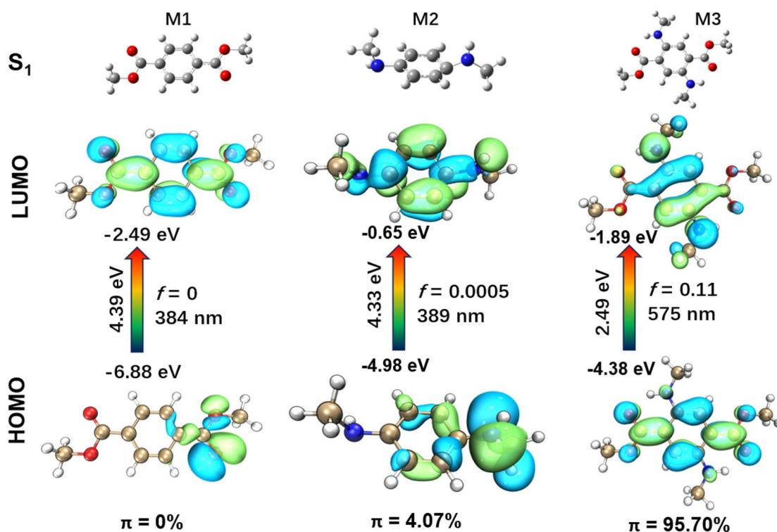
Fig. 4 The molecular configurations and frontier molecular orbitals of three model compounds in the  $S_1$  excited state under gas states, the oscillator strength ( $f$ ) of the  $S_1 \rightarrow S_0$  radiative transition, the theoretical fluorescence emission wavelength, and the percentage of  $\pi$  electrons in the HOMO.
