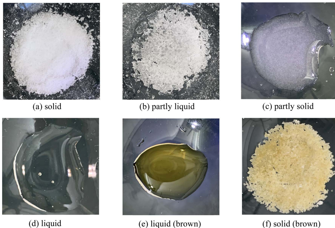
Fig. 1 The pictures of ChCl and glucose mixture after heating at various temperature. (a) Solid: no change, where the mixture retains its white powdered form, (b) partly liquid: partial liquefaction, (c) partly solid: a liquid phase with residual solid particles, (d) liquid: a colorless transparent liquid, (e) liquid (brown): a brown transparent liquid, and (f) solid (brown): a brown solid.
