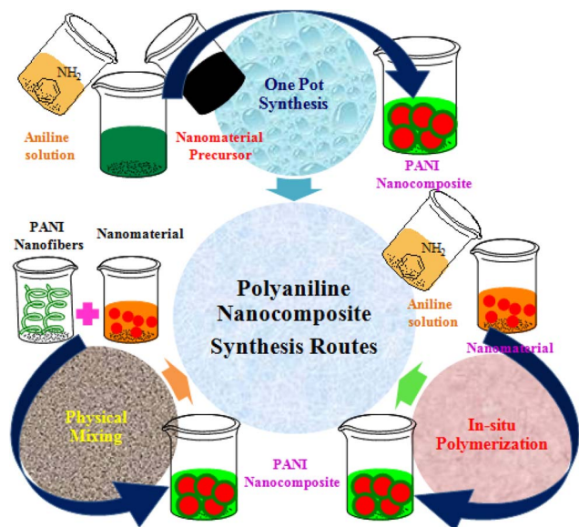
Fig. 2 Polyaniline nanocomposite synthesis routes.
