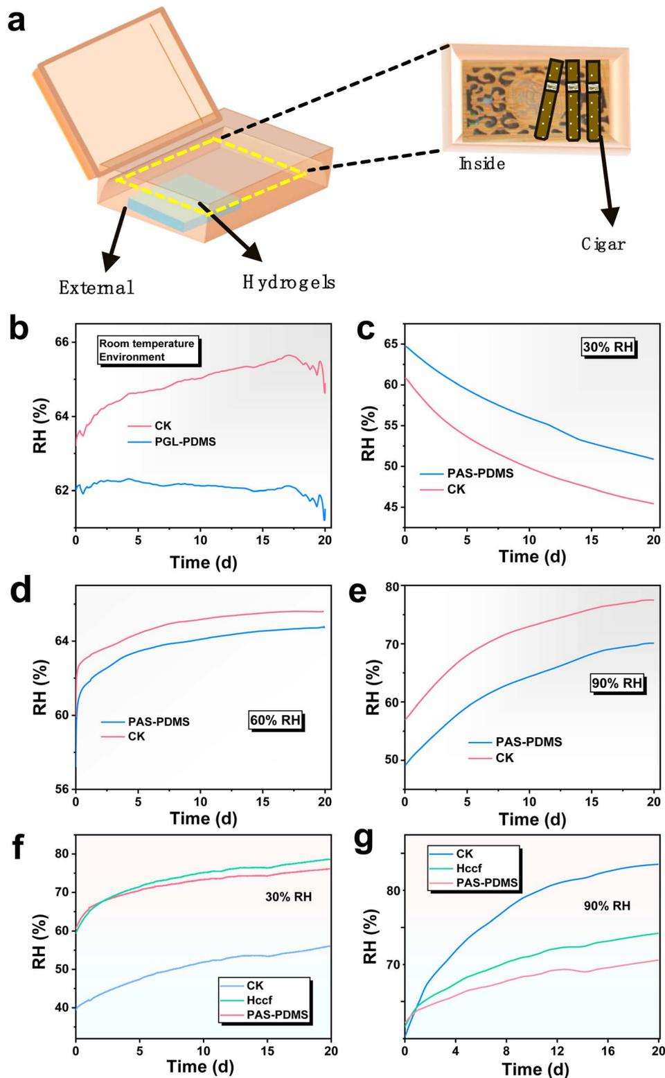
**Fig. 6** (a) Diagram of the PAS-PDMS composite for cigar humidity control. The PAS-PDMS composite's (b) room temperature humidity control curve, (c) 30% RH humidity control curve, (d) 60% RH humidity control curve, (e) 90% RH humidity control curve, (f) comparison of humidity control performance with Hccf under 30% RH conditions, and (g) comparison of humidity control performance with Hccf under 90% RH conditions.
