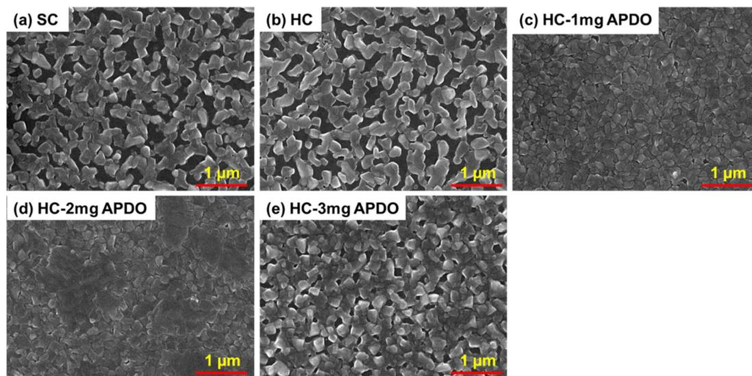
Fig. 5 Surface SEM images of CsPbBr<sub>2.5</sub>Cl<sub>0.5</sub> perovskite films with different preparation methods and APDO doping contents.
