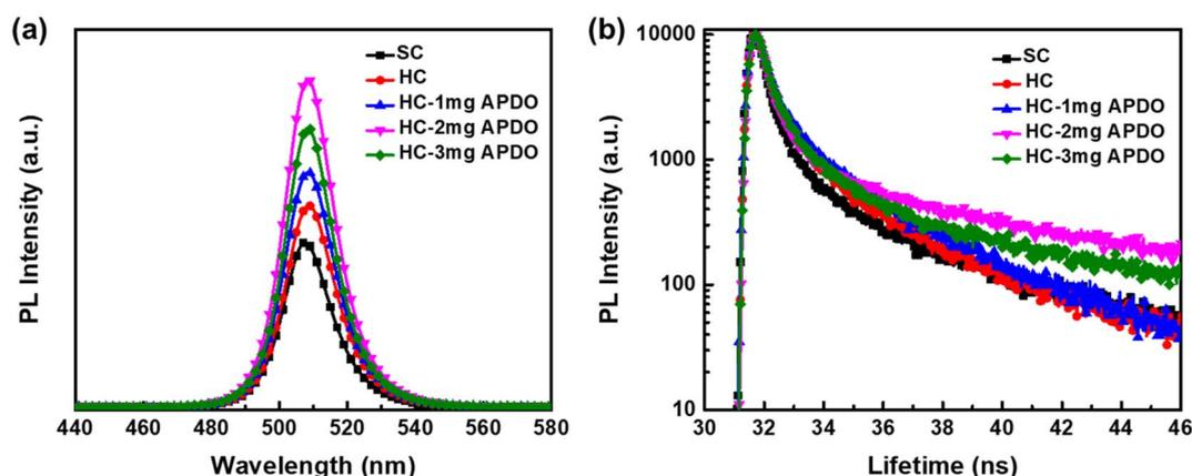
Fig. 2 (a) Photoluminescence (PL), and (b) time-resolved PL spectra of the CsPbBr<sub>2.5</sub>Cl<sub>0.5</sub> perovskite films with different preparation methods and different APDO doping contents.
