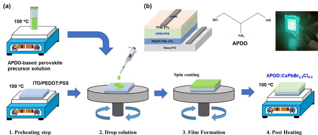
Fig. 1 (a) Schematic of the synthesis route for APDO:CsPbBr<sub>2.5</sub>Cl<sub>0.5</sub> perovskite films. (b) Schematic device structure of PeCLED and luminescence photo.
