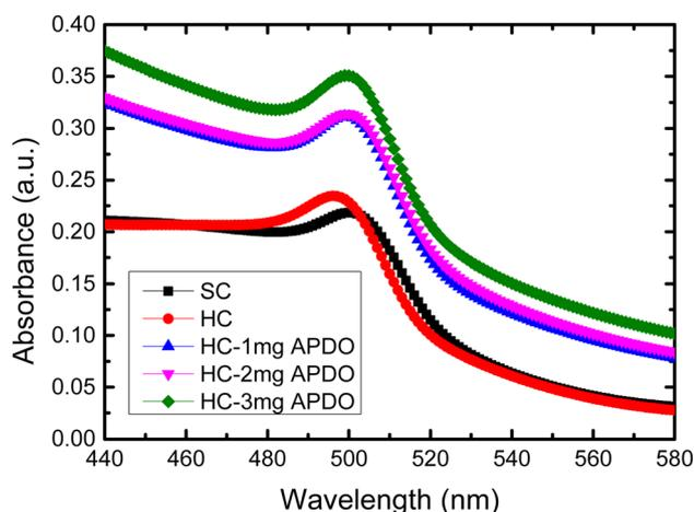
Fig. 3 Absorption spectra of CsPbBr<sub>2.5</sub>Cl<sub>0.5</sub> perovskite films with different preparation methods and different APDO doping contents.
