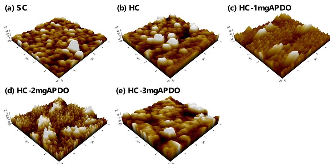
Fig. 6 AFM images of CsPbBr<sub>2.5</sub>Cl<sub>0.5</sub> perovskite films with different preparation methods and APDO doping contents.
