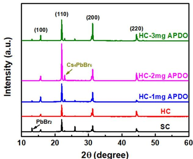
Fig. 4 XRD patterns of CsPbBr<sub>2.5</sub>Cl<sub>0.5</sub> perovskite films with different preparation methods and APDO doping contents.
