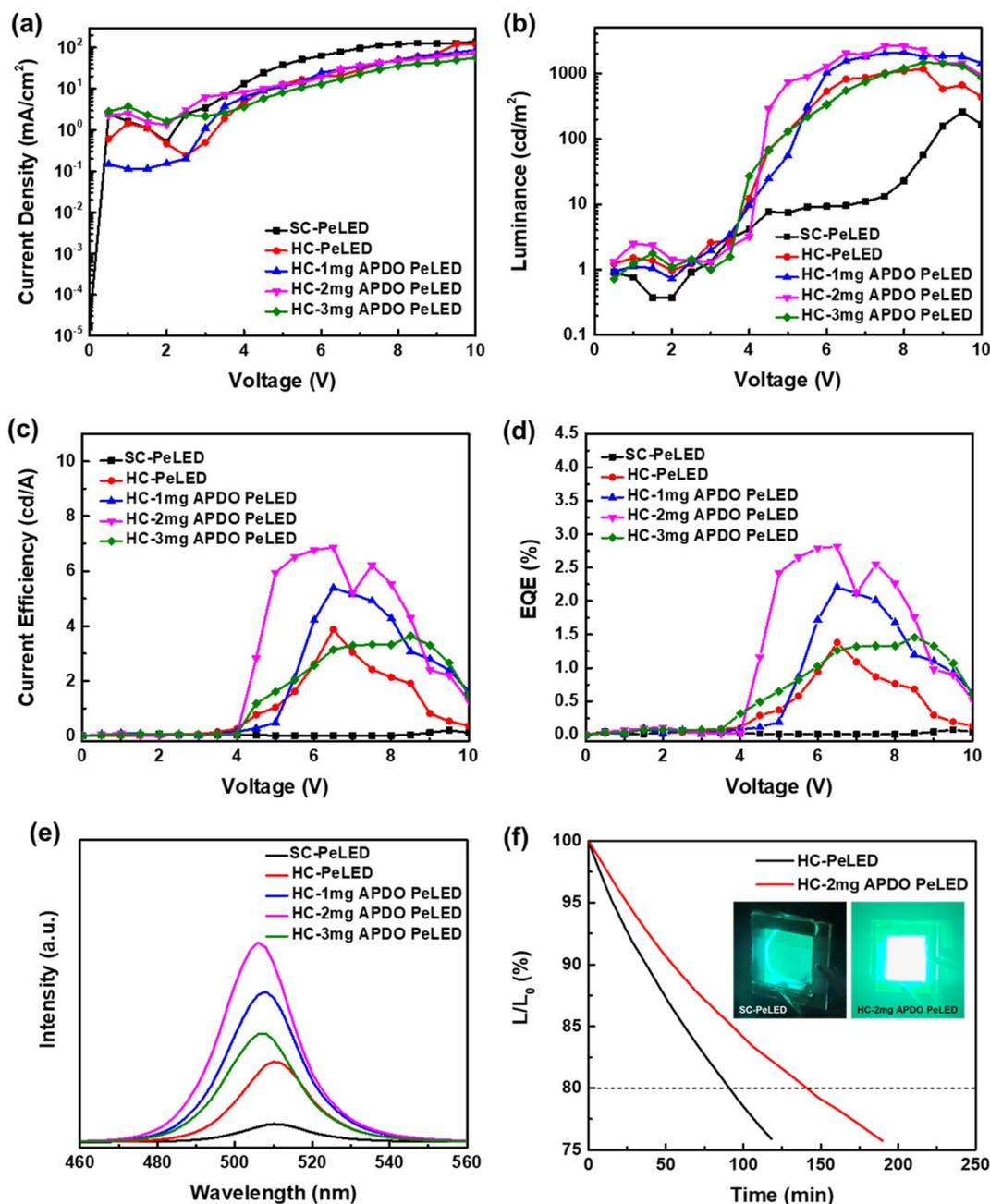
Fig. 7 Characteristics of large-area PeLEDs with different preparation methods and APDO doping contents. (a)  $J$ - $V$ , (b)  $L$ - $V$ , (c)  $CE$ - $V$ , (d)  $EQE$ - $V$ , (e) EL spectra, and (f) operating lifetime test ((inset) photographs of the working SC- and HC-2mg APDO PeLEDs).
