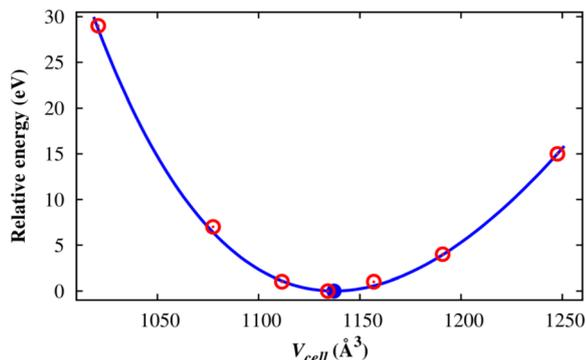
Fig. 2 The total energy (eV) of the  $M(\text{BDC})(\text{TED})_{0.5}$  unit cell as a function of the unit cell volume: calculated values (red points) and the Murnaghan fitting (solid line). The blue point denotes the minimum of the fitted curve.
