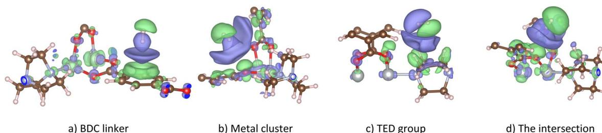
Fig. 6 The charge density difference of  $H_2@Ni(BDC)(TED)_{0.5}$  at the favourable adsorption sites (iso-surface level at  $8 \times 10^{-5} e^- \text{ Bohr}^{-3}$ ): BDC linker (a), metal cluster (b), TED group (c), and the intersection (d). Purple and green present negative charge gain and loss, respectively. Similar characteristics of the charge density difference were also found for the other metal substitutions.
