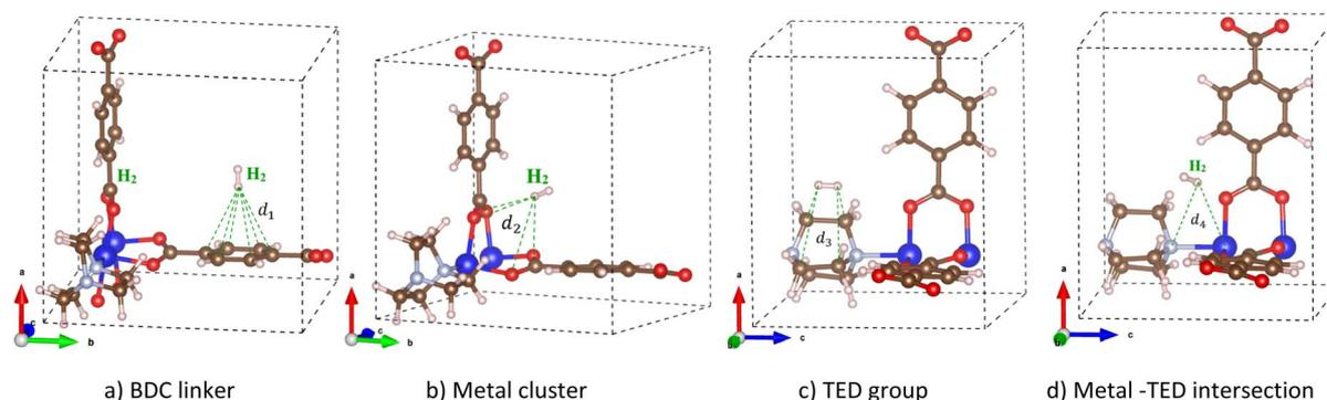
Fig. 3 The favourable adsorption sites of the  $\text{H}_2$  molecule in  $M(\text{BDC})(\text{TED})_{0.5}$  and the denotation for the distances from the nearest H atom of the  $\text{H}_2$  molecule to the neighbouring atoms of  $M(\text{BDC})(\text{TED})_{0.5}$  at the adsorption site: (a) BDC linker, (b) metal cluster, (c) TED group, and (d) the metal cluster-TED intersection.
