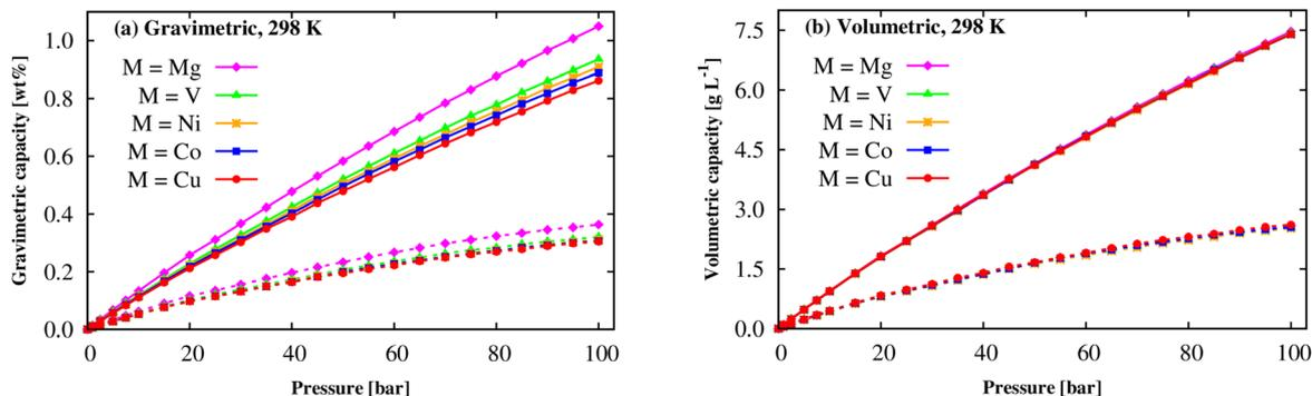
Fig. 8 The H<sub>2</sub> adsorption isotherms of the M(BDC)(TED)<sub>0.5</sub> MOF at 298 K: gravimetric loading (a) and volumetric loading (b). The solid and dashed lines present the absolute ( $n_{\text{abs}}$ ) and excess ( $n_{\text{exc}}$ ) loadings, respectively.
