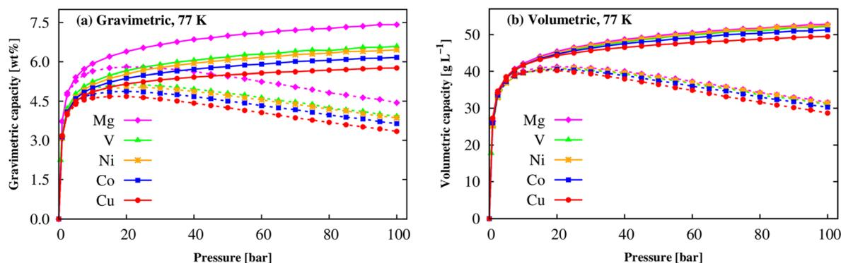
Fig. 9 The  $\text{H}_2$  adsorption isotherms of the  $\text{M}(\text{BDC})(\text{TED})_{0.5}$  MOFs at 77 K: gravimetric uptake (a) and volumetric uptake (b). The solid and dashed lines present the absolute and excess uptakes, respectively.
