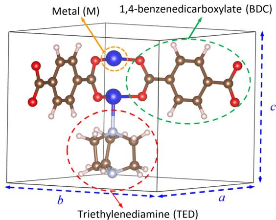
Fig. 1 The primitive unit cell of M(BDC)(TED)<sub>0.5</sub>. Light pink (H), brown (C), light grey (N), red (O), and blue (M).
