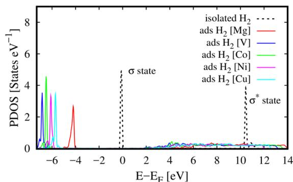
**Fig. 4** The total DOS of the adsorbed hydrogen molecule (ads H<sub>2</sub>) in M(BDC)(TED)<sub>0.5</sub> (M = Mg, V, Co, Ni, and Cu) in the most favourable adsorption configuration (the metal cluster–TED intersection site) and that of the isolated H<sub>2</sub>.
