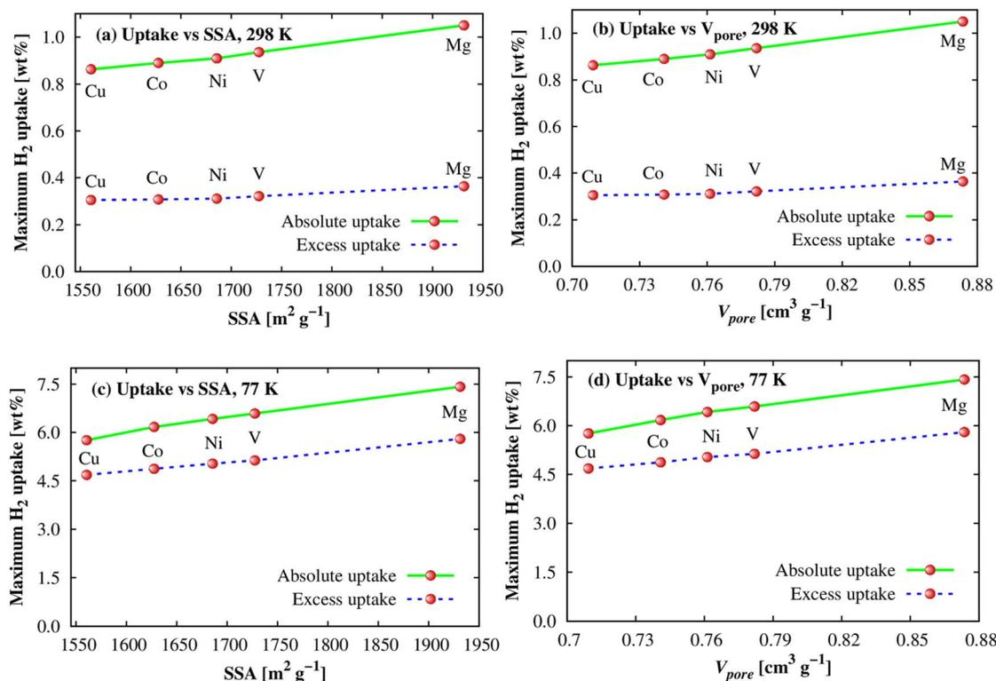
Fig. 10 The dependence of the H<sub>2</sub> gravimetric uptakes on SSA and pore volume of M-MOFs at 298 K (a and b) and 77 K (c and d).
