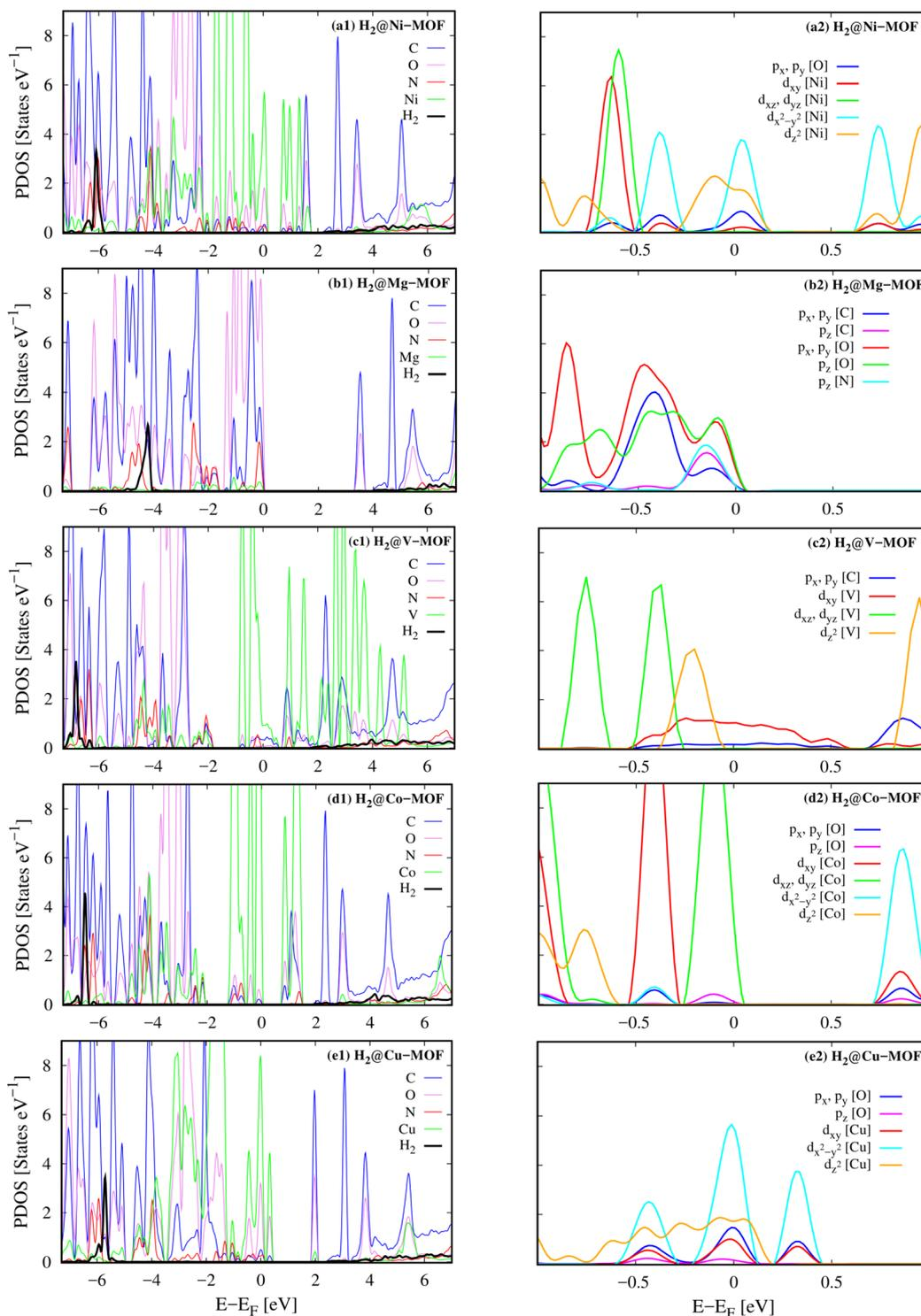
Fig. 5 Left column: the atom-projected DOS of the  $\text{H}_2\text{@M}(\text{BDC})(\text{TED})_{0.5}$  systems (a1–e1). Right column: the orbital-projected DOS around the Fermi level of the adsorbed-state  $\text{M}(\text{BDC})(\text{TED})_{0.5}$  systems (a2–e2) for the metal cluster–TED intersection adsorption site of  $\text{H}_2$ . The identical orbitals are presented with the same colour.
