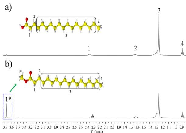
**Fig. 1** <sup>1</sup>H NMR spectra: (a) stearic acid (SA) used as a reagent in the esterification reaction, and (b) methyl stearate (MST) produced in the reaction of SA with methanol.
