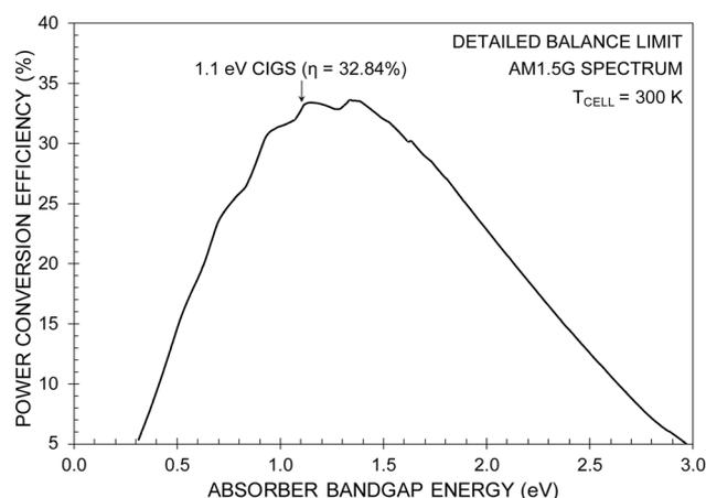
Fig. 2 Detailed balance-limiting power conversion efficiency.
