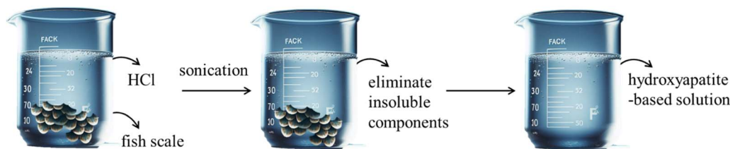
Scheme 1 Preparation of the FHAP solution (fish scale hydroxyapatite-based solution).
