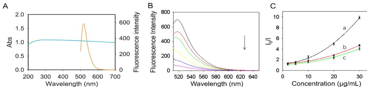
Fig. 2 (A) UV-vis adsorption spectrum (blue line) of BQNPs, and fluorescence emission spectrum of fluorescein (orange line). (B) Fluorescence spectra of fluorescein ( $1.3 \times 10^{-8}$  M) in water with different concentrations of BQNPs (0, 2, 5, 10, 20, 30  $\mu\text{g mL}^{-1}$ , from top to bottom). (C) Stern–Volmer plots of BQNPs (2, 5, 10, 20, 30  $\mu\text{g mL}^{-1}$ ) prepared at varying temperatures, 400 °C (curve a), 600 °C (curve b), and 800 °C (curve c).
