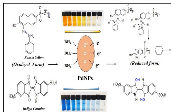
Fig. 16 Possible mechanism of degradation of sunset yellow and indigo carmine by NaBH 4 with PdNPs catalyst.
