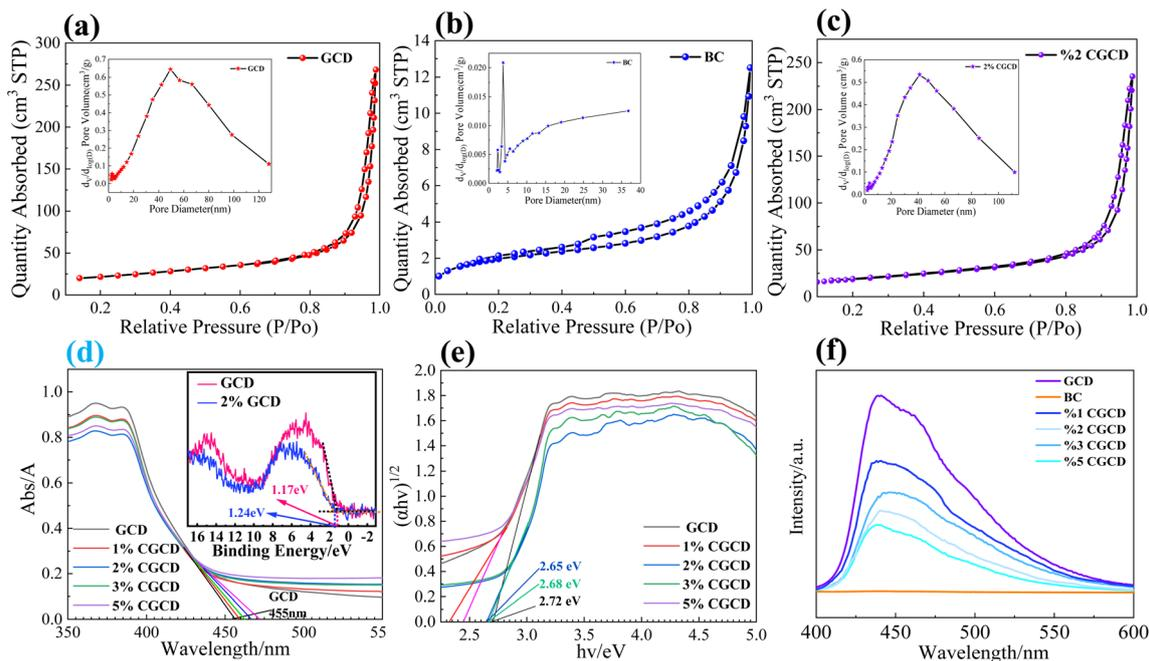
Fig. 6 N<sub>2</sub> isothermal adsorption–desorption curves and pore size distribution of different samples: GCD (a); BC (b); 2% CGCD (c). UV-vis spectra and valence band spectrum of different samples (d); Tauc-curve (e); PL spectra (f).
