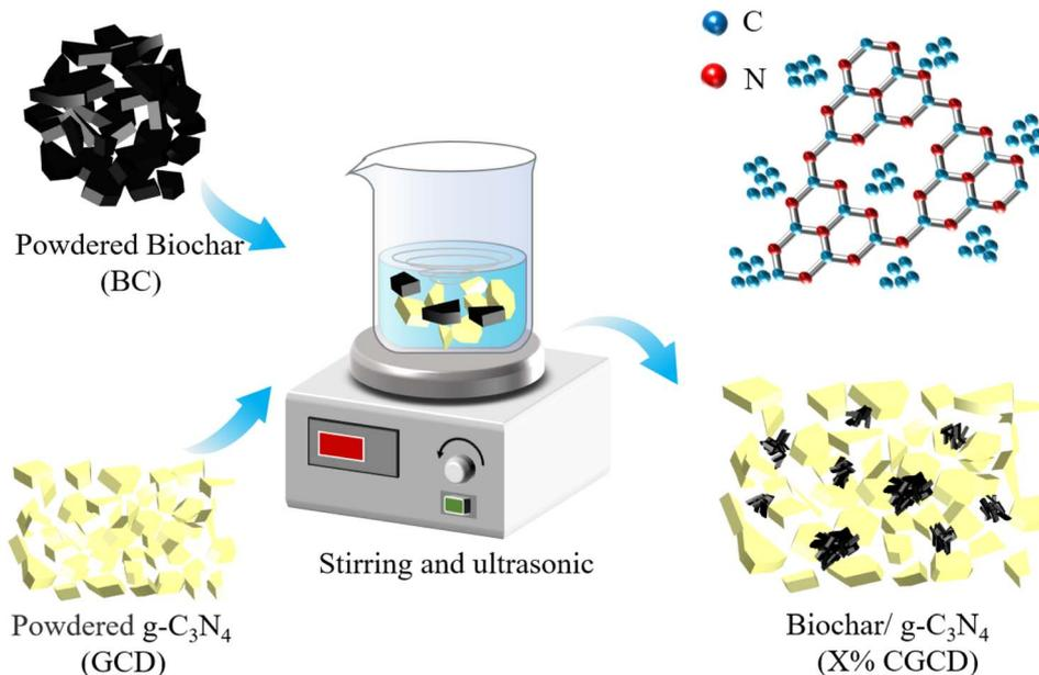
Fig. 1 Flow chart for the preparation of CGCD.
