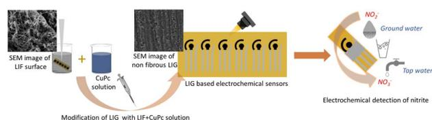
Fig. 1 Graphical illustration of (a) the sonication of LIF electrodes for the dispersion and preparation of the composite of LIF and CuPc, (b) fabrication of LIG electrodes by  $\text{CO}_2$  laser and modification with the composite by drop-casting on the surface, and (c) electrochemical detection of nitrite in ground, drinking, and tap water.
