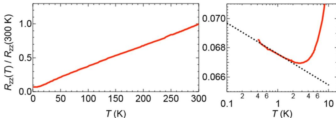
Fig. 8 Electric resistance of  $\beta''$ -(BEDT-TTF)<sub>4</sub>[(H<sub>3</sub>O)Cr(C<sub>2</sub>O<sub>4</sub>)<sub>3</sub>]·phenol (II). The upturn in resistance below 10 K is shown on the right-hand side.
