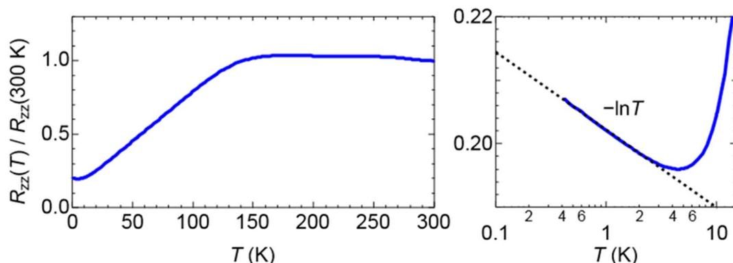
Fig. 9 Electrical resistance of  $\beta''$ -(BEDT-TTF)<sub>4</sub>[(H<sub>3</sub>O)Cr(C<sub>2</sub>O<sub>4</sub>)<sub>3</sub>]·salicylaldehyde (III). The upturn in resistance below 10 K is shown on the right-hand side.
