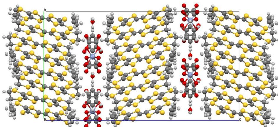
Fig. 5 Layered packing of  $\beta''$ -(BEDT-TTF)<sub>4</sub>[(H<sub>3</sub>O)Cr(C<sub>2</sub>O<sub>4</sub>)<sub>3</sub>]·phenol (II) viewed down the *a* axis.
