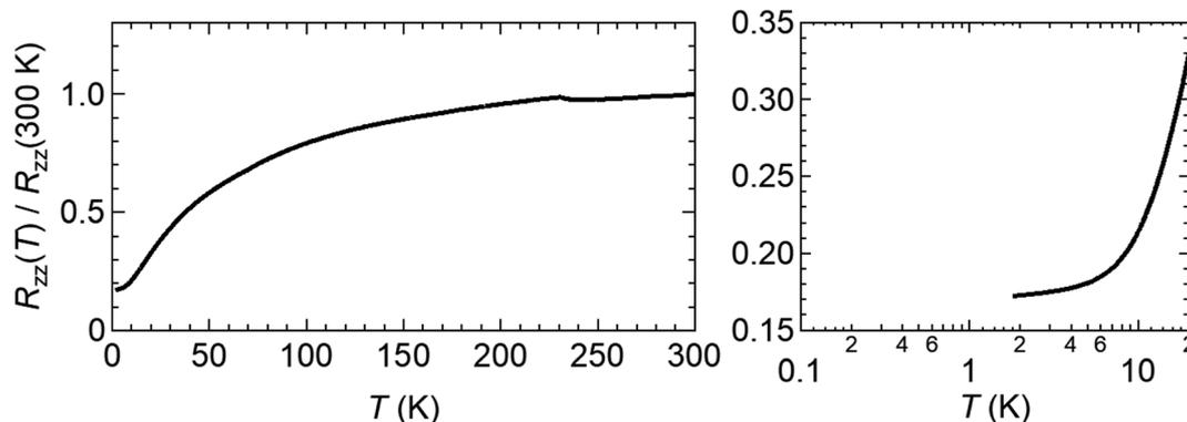
Fig. 4 Electrical resistance of  $\beta''$ -(BEDT-TTF)<sub>4</sub>[(NH<sub>4</sub>)Cr(C<sub>2</sub>O<sub>4</sub>)<sub>3</sub>]·toluene (I). The resistance below 10 K is shown on the right-hand side.
