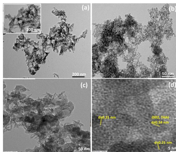
Fig. 2 TEM images of the (a) multi-trace elements co-doped apatite ( $\text{Ca}_{10-\delta}\text{M}_\delta(\text{PO}_4)_{5.5}(\text{CO}_3)_{0.5}(\text{OH})_2$ , M = trace elements, THA), (b) magnetic Mn–Zn nanoferrite ((Mn, Zn) $\text{Fe}_2\text{O}_4$  particles, BioMags) and THAiBioMags nanoparticles at low (c) and high (d) resolution, respectively.
