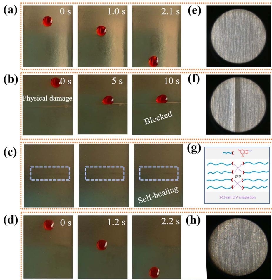
Fig. 4 Motion of a water droplet (20  $\mu$ L) on the original SMEMG (a), SMEMG damaged via scalpel scratching, (b) and a self-healed SMEMG surface (d) under 365 nm UV light irradiation for 3 h; (c) a self-healed SMEMG surface under 365 nm UV light irradiation for 3 h. Optical microscopy images of original SMEMG (e), damaged SMEMG (f) and self-healed SMEMG surface (h). (g) Self-healing mechanism of damaged SMEMG under 365 nm UV light irradiation. The water droplet was dyed with methyl orange.
