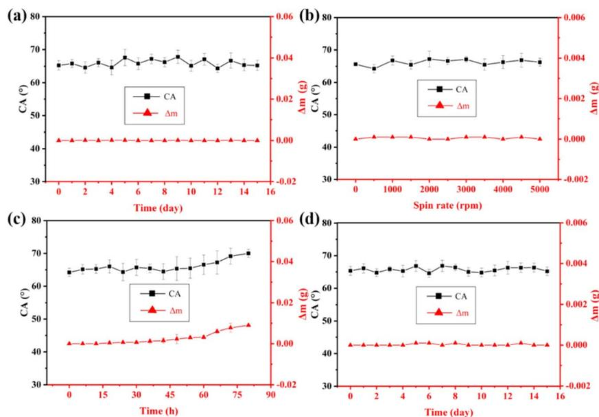
Fig. 6 Durability of the SMEMG. Variation of the CA and  $\Delta m$  of the SMEMG during the stability test. (a) SMEMG after heating at  $80^\circ\text{C}$  for 1–15 days; (b) SMEMG rotated at 0–5000 rpm for 1 min; (c) SMEMG after immersing in water with a spin rate of 30 rpm for 80 h; (d) SMEMG placed in the vertical position for 1–15 days.
