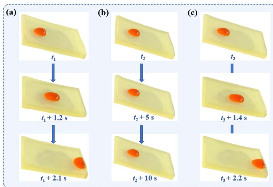
Fig. 7 Dynamic control of the mobility of a water droplet (20  $\mu$ L) on the SMEMG. (a) Process of a water droplet slipping off the SMEMG at the initial state. (b) Process of a water droplet pinned on the SMEMG after the surface lubricant oil was swabbed. (c) Process of a water droplet re-sliding down the SMEMG after UV irradiation for 3 h.
