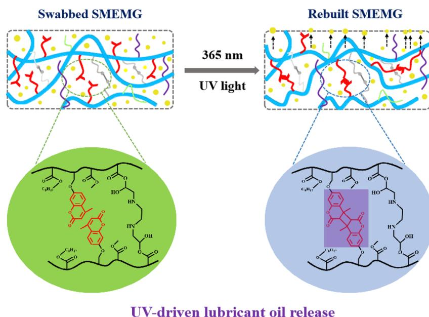
**Fig. 9** Lubricant oil self-replenishing mechanism of the SMEMG.
