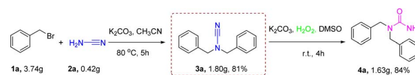
Scheme 4 Gram-scale synthesis of 4a . Conditions of reaction: 1a (22.0 mmol), 2a (10.0 mmol), K_2CO_3 (30.0 mmol) in MeCN (25 mL) stirred for 5 h at 80 °C under air atmosphere, isolated yields; 3a (8.1 mmol), H_2O_2 (9.7 mmol), K_2CO_3 (8.1 mmol) in DMSO (15 mL) stirred for 4 h at r.t. under air, isolated yields.
