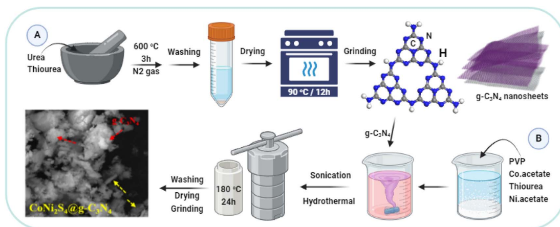
Fig. 1 Schematic design for g\text{-C}_3\text{N}_4 (A) and \text{CoNi}_2\text{S}_4@g\text{-C}_3\text{N}_4 synthesis (B).
