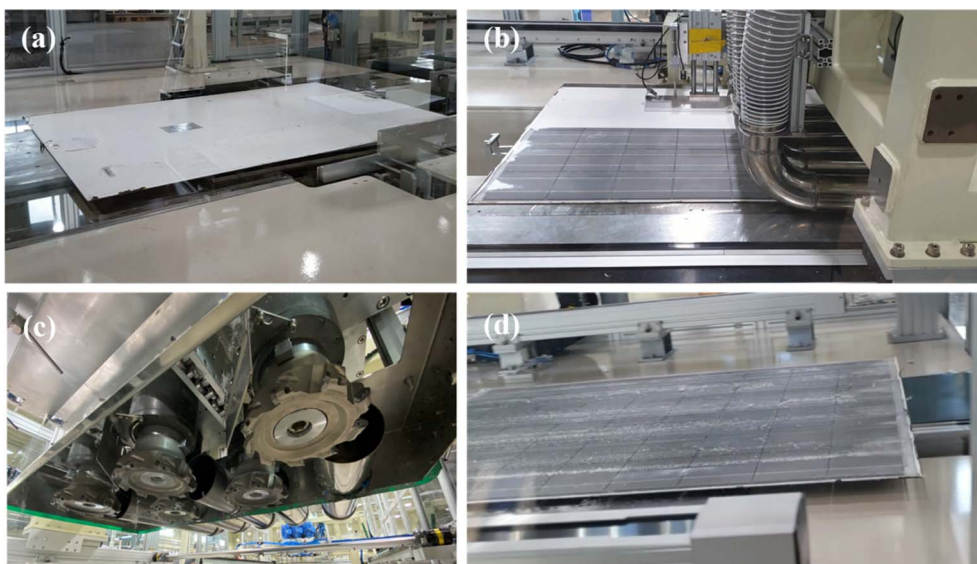
Fig. 2 Process overview of the back-sheet, (a) Al frame and junction box removed PV module, (b) automatic transfer PV modules, (c) image of T-cutter of the back-sheet removal equipment and (d) PV module after back-sheet removal process.
