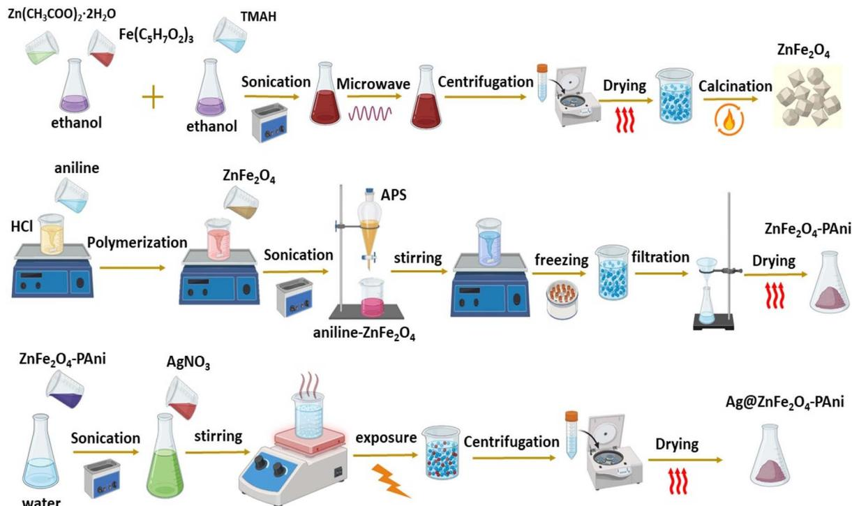
Fig. 1 Schematic diagram for preparation of Ag@ZnFe<sub>2</sub>O<sub>4</sub>-PANI nanocomposite.
