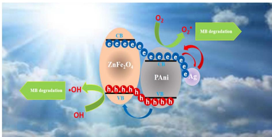
Fig. 11 Schematic view for possible photocatalytic mechanism behind Ag@ZnFe<sub>2</sub>O<sub>4</sub>-PANI nanocomposites for photo-degradation of dye molecules.
