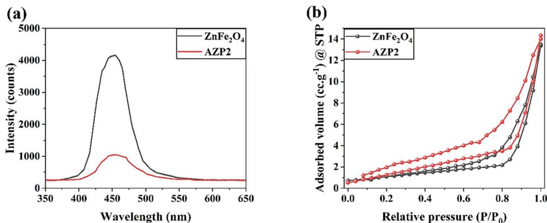
Fig. 7 (a) PL spectra and (b) BET curves of ZnFe<sub>2</sub>O<sub>4</sub> and AZP2 nanostructures.
