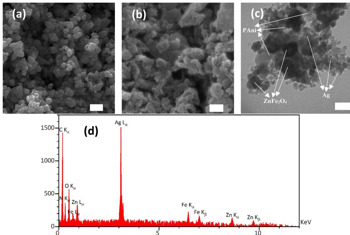
Fig. 4 FESEM image of (a)  $\text{ZnFe}_2\text{O}_4$  and (b) AZP2. TEM image of (c) AZP2. (d) EDS elements mapping images of AZP2 composite. Scale bar of FESEM and TEM images are 200 nm and 80 nm, respectively.
