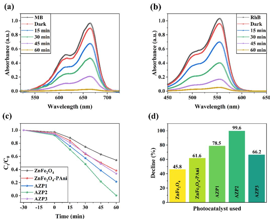
Fig. 8 Photocatalytic activity of AZP2 for (a) MB and (b) RhB dyes. (c) Kinetic plot versus illumination time for MB of ZnFe<sub>2</sub>O<sub>4</sub>, ZnFe<sub>2</sub>O<sub>4</sub>-PANi, AZP1, AZP2, and AZP3 nanostructures. (d) Comparison of MB degradation over different photocatalyst.
