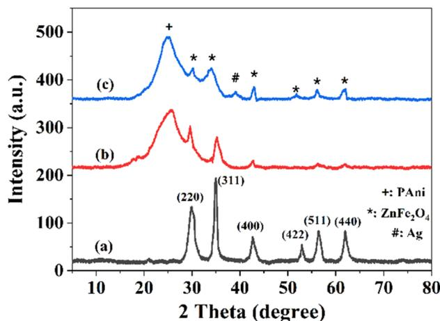
Fig. 2 XRD spectra of (a) ZnFe<sub>2</sub>O<sub>4</sub>, (b) ZnFe<sub>2</sub>O<sub>4</sub>-PANI, and (c) AZP2 nanostructures.
