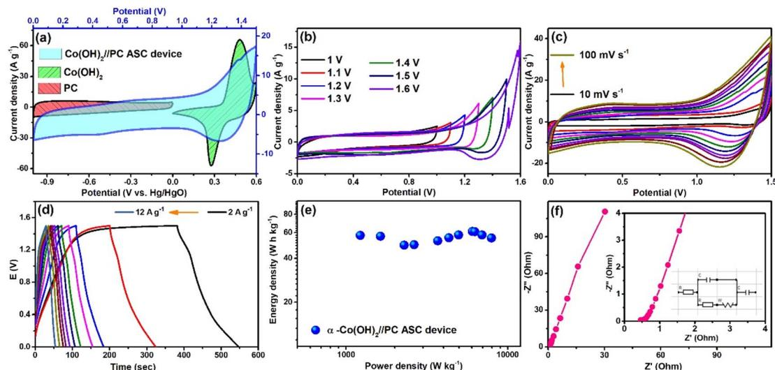
Fig. 5 (a) CV curves of  $\text{Co}(\text{OH})_2$  (0–0.6 V), PC (–1–0 V), and  $\text{Co}(\text{OH})_2//\text{PC}$  ASC devices (0–1.5 V) at a scan rate of  $30 \text{ mV s}^{-1}$ . (b) CV curves with different potential window, (c) CV curves with different scan rates, (d) GCD profile with different current densities, (e) Ragone plot, and (f) Nyquist plot (inset: Nyquist plot in the high-frequency region and fitted circuit) of the  $\text{Co}(\text{OH})_2//\text{PC}$  ASC device.
