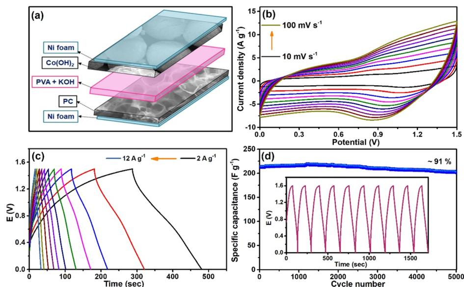
Fig. 6 (a) Graphical sketch of a solid-state  $\text{Co}(\text{OH})_2//\text{PC}$  ASC device. (b) CV scans and (c) GCD curves of the solid-state  $\text{Co}(\text{OH})_2//\text{PC}$  ASC device. (d) Cycling stability test (inset: first GCD 10 cycles) of the device.
