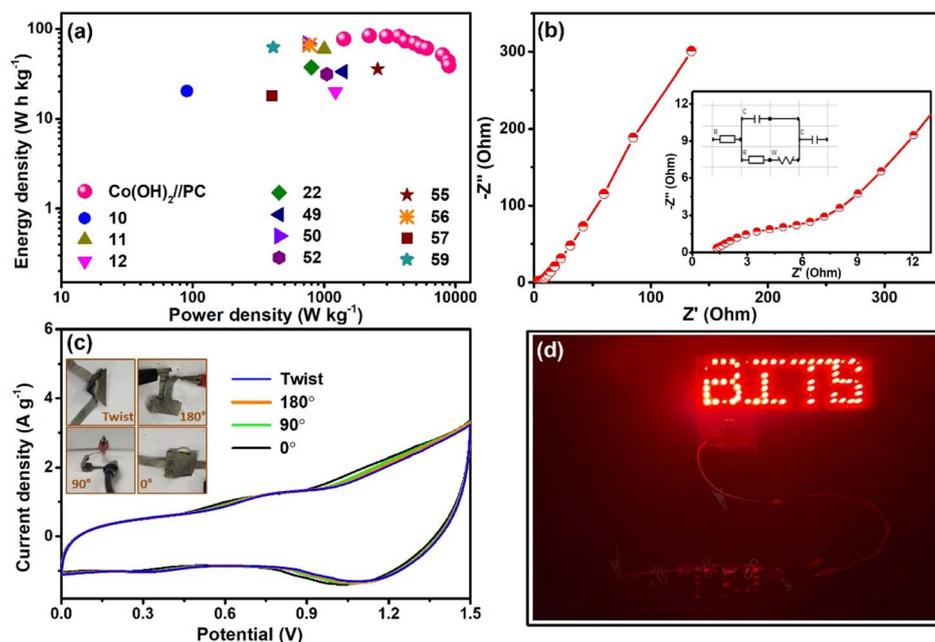
Fig. 7 (a) Ragone plot of the solid-state  $\text{Co(OH)}_2//\text{PC}$  ASC device with a comparison of reported research on  $\text{Co(OH)}_2$ -based supercapacitors, (b) Nyquist plot, and (c) CV test with different angles of the solid-state ASC device. (d) LED light illuminated by the solid-state ASC device.
