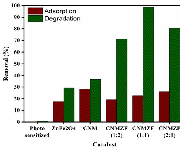
Fig. 1 Adsorption and photocatalytic removal of CR dye ( $10 \text{ mg L}^{-1}$ ) with different CNMZF compositions compared to bare photocatalysts, conducted under dark and visible light (50 W) conditions for 75 minutes.
