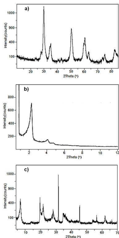
Fig. 1 XRD patterns of (a) SZ, (b) Al-MCM-41 and (c) montmorillonite modified with CF<sub>3</sub>SO<sub>3</sub>H.
