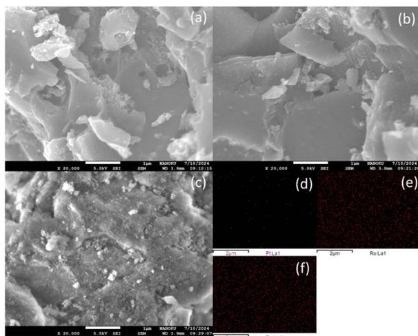
Fig. 3 SEM-DES of catalysts (a) Pt/C, (b) Ru/C, (c) Ru/Al<sub>2</sub>O<sub>3</sub>, (d) Pt particles on C, (e) Ru particles on C and (f) Ru particles on Al<sub>2</sub>O<sub>3</sub>.
