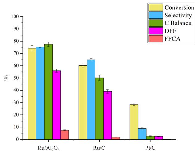
Fig. 5 Impact of catalyst types on reaction performance. Experimental conditions: temperature maintained at 120 °C, 5-HMF solution concentration of 5 g L<sup>-1</sup>, flow rate of 0.06 ml min<sup>-1</sup> for 5-HMF solution, acetonitrile utilized as the solvent, oxygen gas flow rate set at 10 ml min<sup>-1</sup>, and catalyst quantity of 0.05 g.
