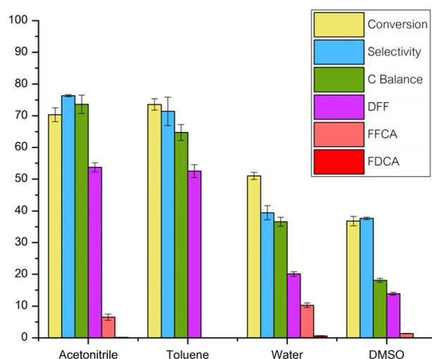
Fig. 6 Impact of solvent on reaction performance. Experimental conditions: temperature maintained at 120 °C, 5-HMF solution concentration of 5 g L<sup>-1</sup>, flow rate of 0.06 ml min<sup>-1</sup> for 5-HMF solution, oxygen gas flow rate set at 10 ml min<sup>-1</sup>, and catalyst quantity of 0.05 g (Ru/Al<sub>2</sub>O<sub>3</sub>).
