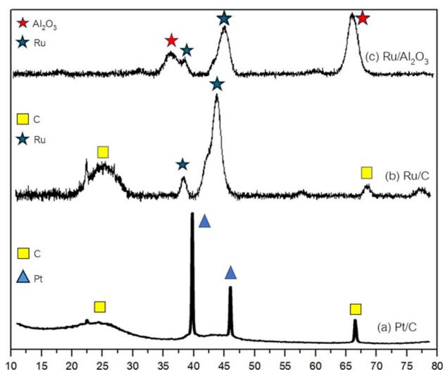
Fig. 2 The XRD pattern of catalyst (a) Pt/C, (b) Ru/C and (c) Ru/Al<sub>2</sub>O<sub>3</sub>.
