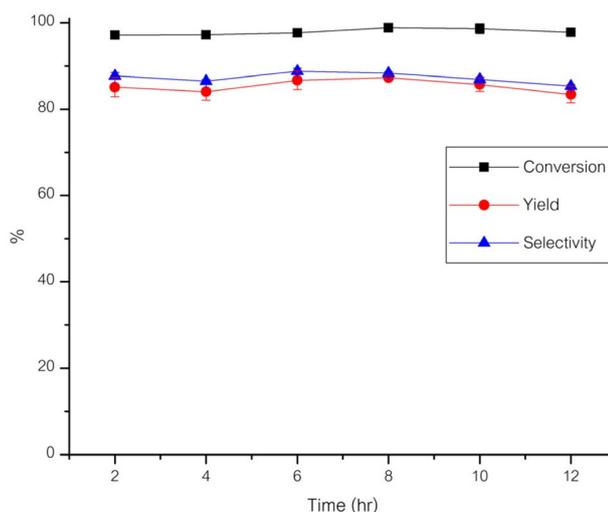
Fig. 10 Reaction performance of DFF synthesis over Ru/Al<sub>2</sub>O<sub>3</sub> catalyst over an extended period.
