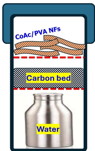
Fig. 1 Schematic diagram for the used reactor for preparation the organic cobalt nanofibers.
