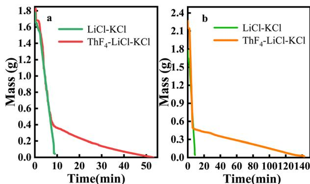
Fig. 2 Mass loss curves under vacuum distillation conditions at 1173 K and 20 Pa: (a) 1.8 g of 20 wt% ThF<sub>4</sub>–LiCl–KCl and 1.8 g of LiCl–KCl; (b) 2.25 g of 20 wt% ThF<sub>4</sub>–LiCl–KCl and 1.8 g of LiCl–KCl.
