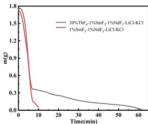
Fig. 7 Weight loss curves of 20 wt% ThF<sub>4</sub>-1 wt% SmF<sub>3</sub>-1 wt% NdF<sub>3</sub>-LiCl-KCl mixed salt.
