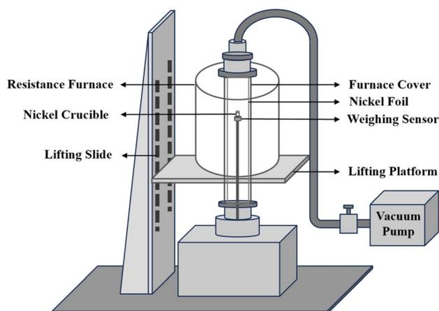
Fig. 1 A Schematic diagram of vacuum distillation apparatus.
