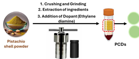
Fig. 1 Schematic of synthesis of PCDs.
