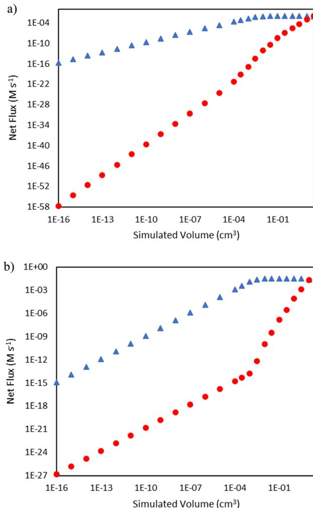
**Fig. 5** Comparison of rates of hydrogen abstraction from ethylene by 1,4-butyl diradical (blue triangles  $\blacktriangle$ ) and butene diradical (red circles  $\bullet$ ) as a function of reactor volume. a) Total pressure 15 bar b) total pressure 25 bar.
