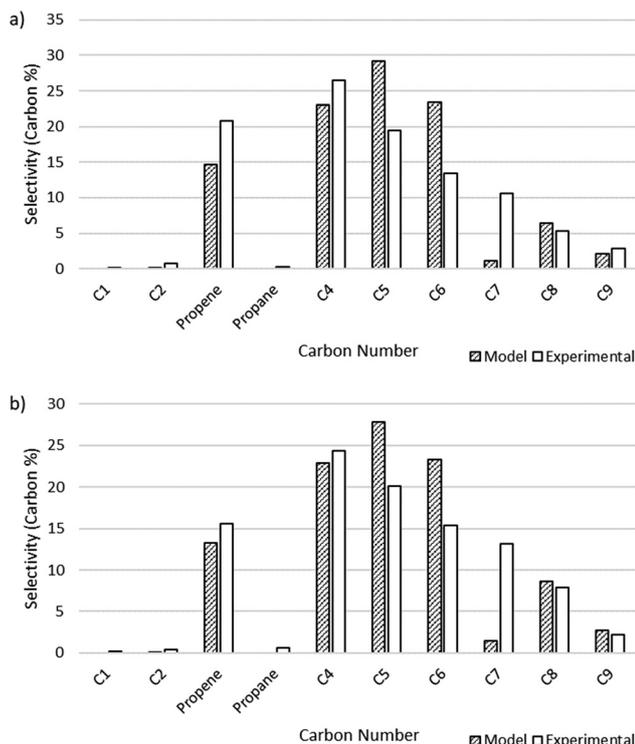
**Fig. 4** Microkinetic model output showing selectivity measured by carbon percent for different carbon number species. a) Total pressure of 15 bar. Model conversion: 20.6%. Experimental conversion: 21%. b) Total pressure of 25 bar. Model conversion: 63.7%. Experimental conversion: 56%.
