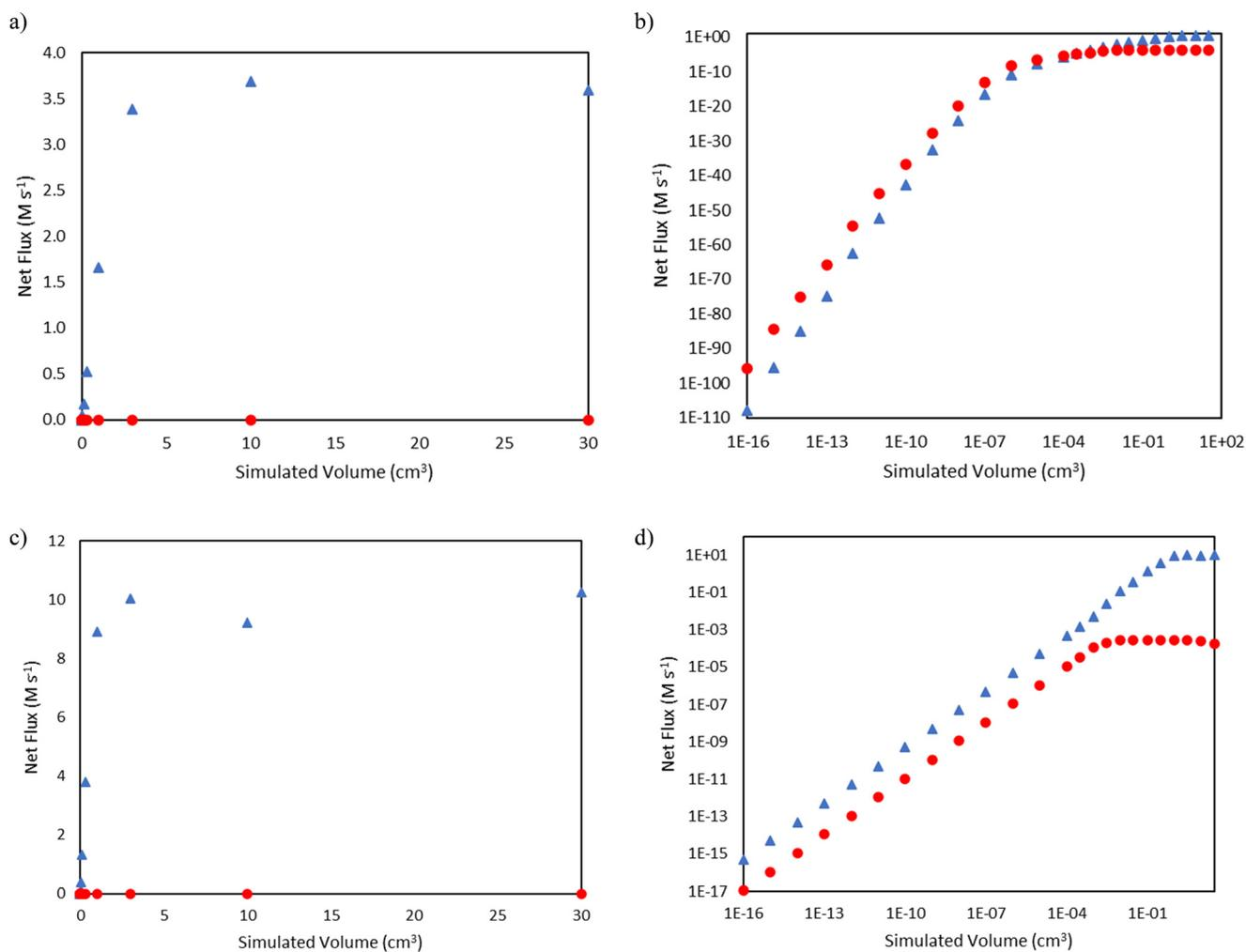
**Fig. 6** Comparisons of net flux of nonenyl  $\beta$ -scission (blue triangles  $\blacktriangle$ ) and nonyl  $\beta$ -scission (red circles  $\bullet$ ) as a function of reactor volume. a) Total pressure 15 bar, linear scale b) total pressure 15 bar, log-log scale c) total pressure 25 bar, linear scale d) total pressure 25 bar, log-log scale.
