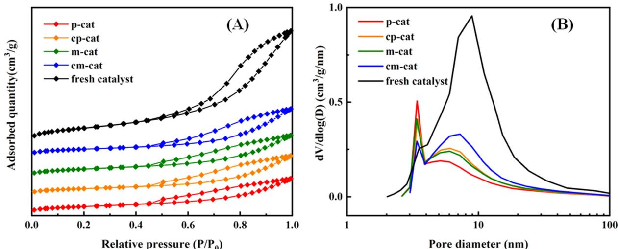
Fig. 5 N<sub>2</sub> adsorption-desorption isotherms (A) and pore size distribution curves (B) calculated from adsorption branches of the fresh catalyst, A2, A3, AC2 and AC3.
