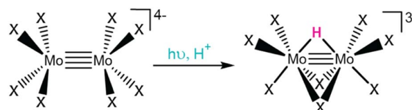
Fig. 6 Excited state protonation of [\text{Mo}_2\text{X}_8]^{4-} yields [\text{Mo}_2(\mu\text{-H})(\mu\text{-X})_2(\text{X})_6]^{3-} .
