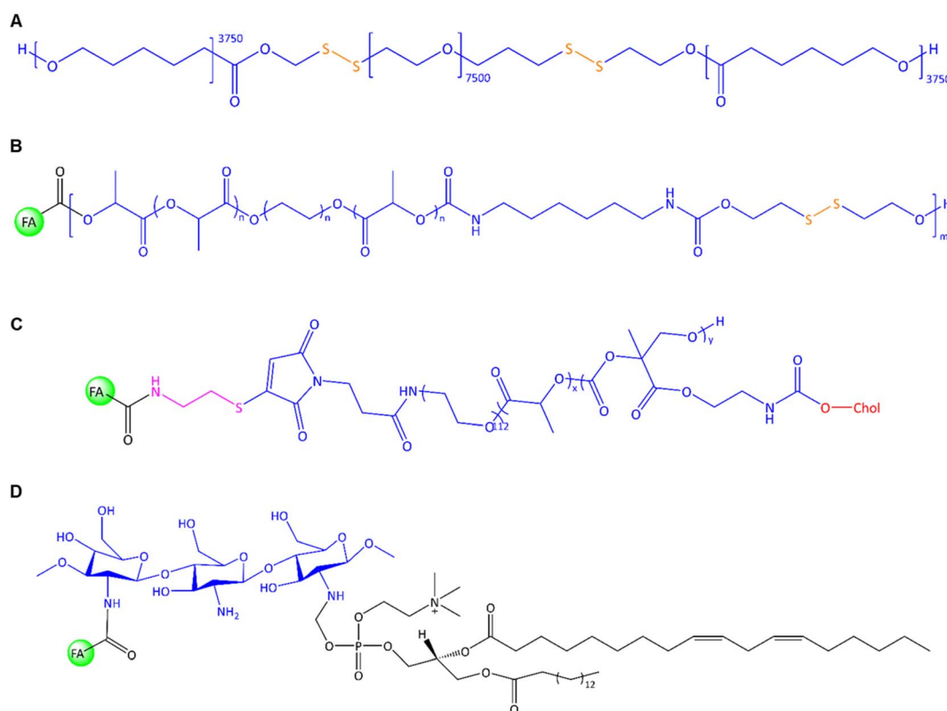
Fig. 9 The chemical structure of (A) PCL-ss-PEG-ss-PCL, (B) FA-conjugated chitosan-lipid NPs, (C) FA-PEG- b-p -(MTC-Chol-co-LA) lipopolymer, (D) FA-conjugated chitosan/phospholipids (lipid S75).
