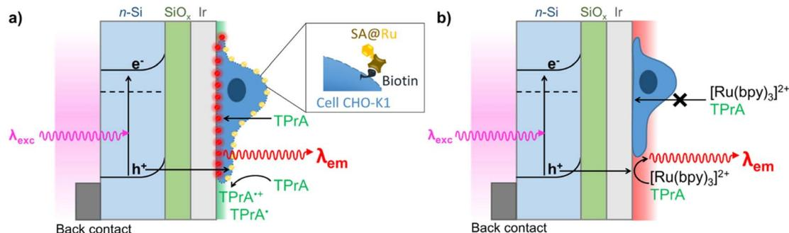
**Fig. 1** Schematic representation of two PECL microscopy modes for imaging single cells with back-illumination configuration. (a) Direct imaging by PECL+ of cell membrane labeled with the streptavidin-modified [Ru(bpy)<sub>3</sub>]<sup>2+</sup> luminophore (SA@Ru) in TPrA solution; and (b) label-free imaging of cells by PECL- with cells immersed in a PBS solution containing both [Ru(bpy)<sub>3</sub>]<sup>2+</sup> and TPrA.
