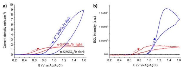
**Fig. 2** (a) Cyclic voltammograms and (b) corresponding ECL signals of n-Si/SiO<sub>x</sub>/Ir in the dark (black curve) or under 1050 nm infrared illumination (red curve) compared to the p<sup>+</sup>-Si/SiO<sub>x</sub>/Ir electrode in the dark (blue curve) in a PBS solution (pH 7.4) containing 30 μM [Ru(bpy)<sub>3</sub>]<sup>2+</sup> and 0.1 M TPrA. Scan rate: 50 mV s<sup>-1</sup>.
