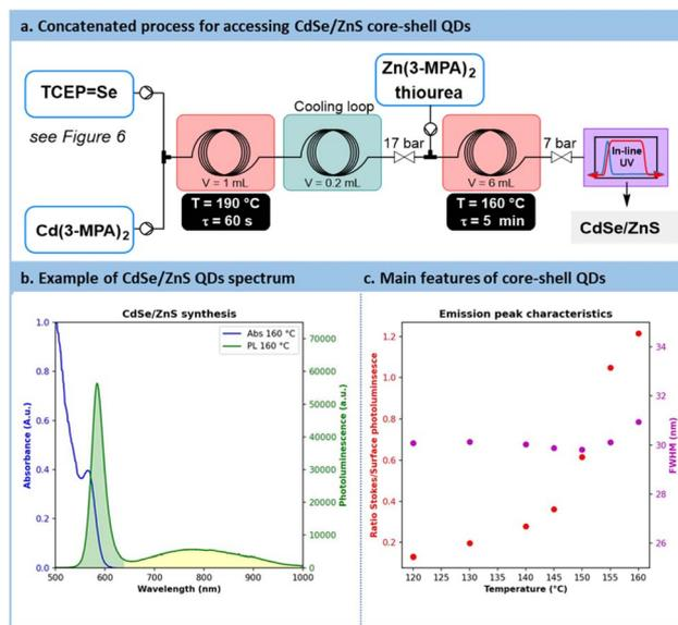
Fig. 9 Passivation of surface trap states through the preparation of CdSe/ZnS core–shell QDs. (a) Concatenated process with the injection of Zn(3-MPA)<sub>2</sub> and thiourea downstream the preparation of CdSe QDs. (b) Absorbance (blue line, A.u. = Absorbance units) and photoluminescence (green line, a.u. = arbitrary unit) of CdSe/ZnS QDs. (c) Effect of the temperature on the ratio fluorescence/surface emission (red scatter) and the peak full width at half maximum (FWHM) (magenta scatter).
