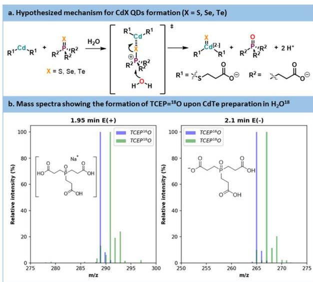
Fig. 10 (a) Hypothesized mechanism for CdX QDs formation. (b) Mass spectra of TCEP=<sup>18</sup>O obtained from synthesis using labelled H<sub>2</sub><sup>18</sup>O and a reference of TCEP=<sup>16</sup>O.
